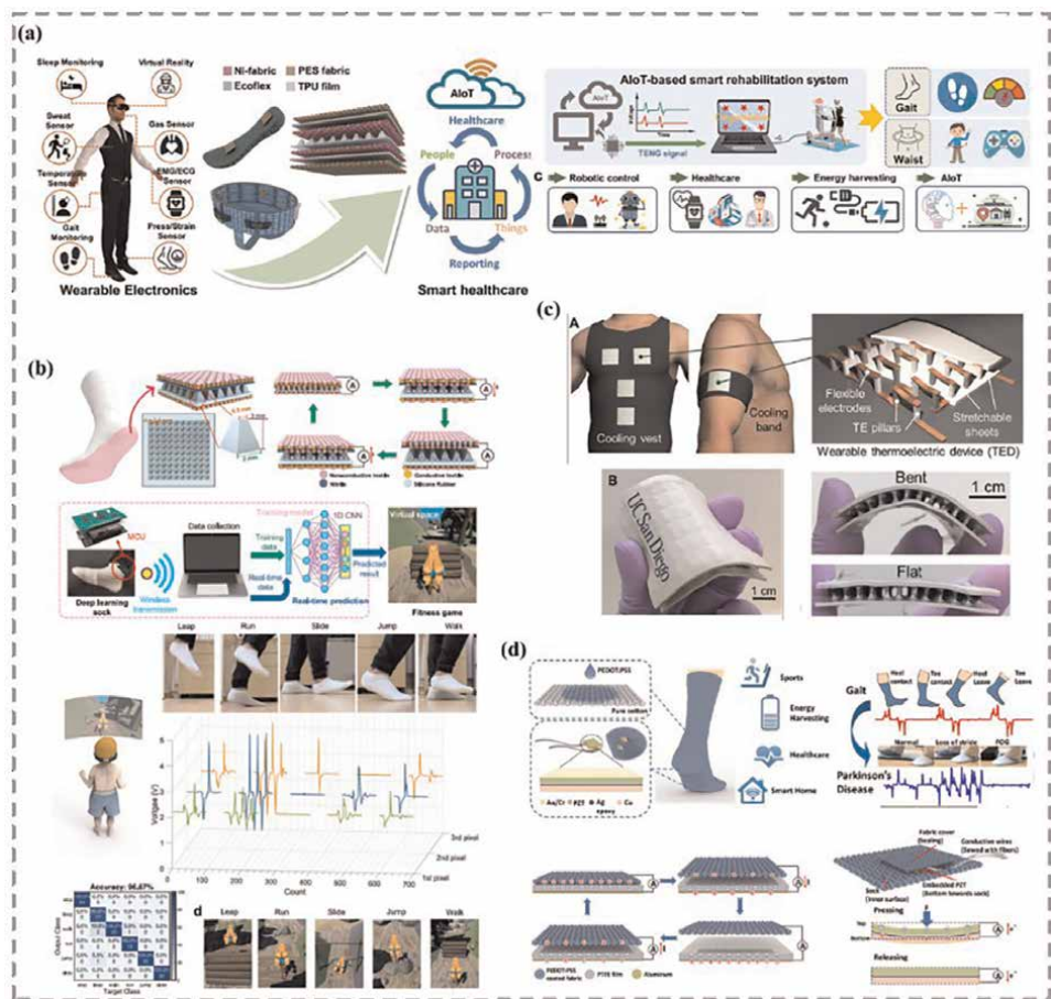
Figure 6. (a) A fabric triboelectric array structure prepared by screen printing using silver paste and carbon nanotube (CNT) ink. Reproduced with permission from Ref. [62] Copyright 2022 Wiley-VCH. (b) A smart sock system with integrated TENG arrays to achieve individual identity recognition and behavior classification. Reproduced with permission from Ref. [63] Copyright 2020 Springer Nature. (c) A flexible thermoelectric device (TED) system for active thermal management in dynamic environments. Reproduced with permission from Ref. [64] Copyright 2019 Science. (d) A fabric-based hybrid nanogenerator used for physiological signal acquisition and personalized rehabilitation training systems. Reproduced with permission from Ref. [65] Copyright 2019 American Chemical Society.
